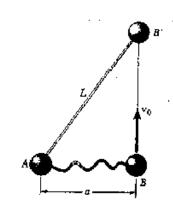
4. A uniform slender rod is placed at corner B and is given a slight clockwise motion. Assuming that the corner is sharp and becomes slightly embedded in the end of the rod, so that the coefficient of static friction at B is very large, determine (a) the angle β through which the rod will have rotated when it loses contact with the corner, (b) the corresponding velocity of end A. (25%)
